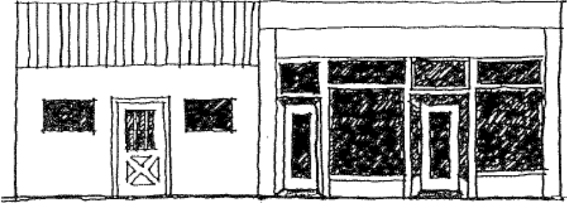
NO. INSUFFICIENT WINDOW OPENINGS.
